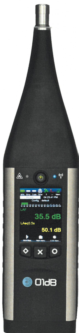
Abb. 1: FUSION Smart Sound & Vibration Analyzer
